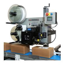
simultaneously print and apply variableimprint or blank labels to the tops, bottoms or sides of products right along the conveyor line.
